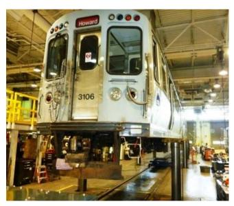
Skokie Shop staff. All of the 256 cars have undergone the base overhaul as of October 31, 2018. There has been an increase in the scope of repairs based on car condition observed during the program. CTA brought the required cars back for the work remaining and completed the overhaul in December 2018.
