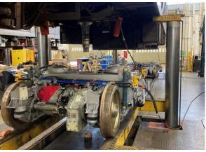
Installation of a new truck assembly on the 5000-series rail car.
