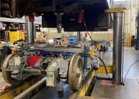
Installation of a new truck assembly on the 5000-series rail car.
