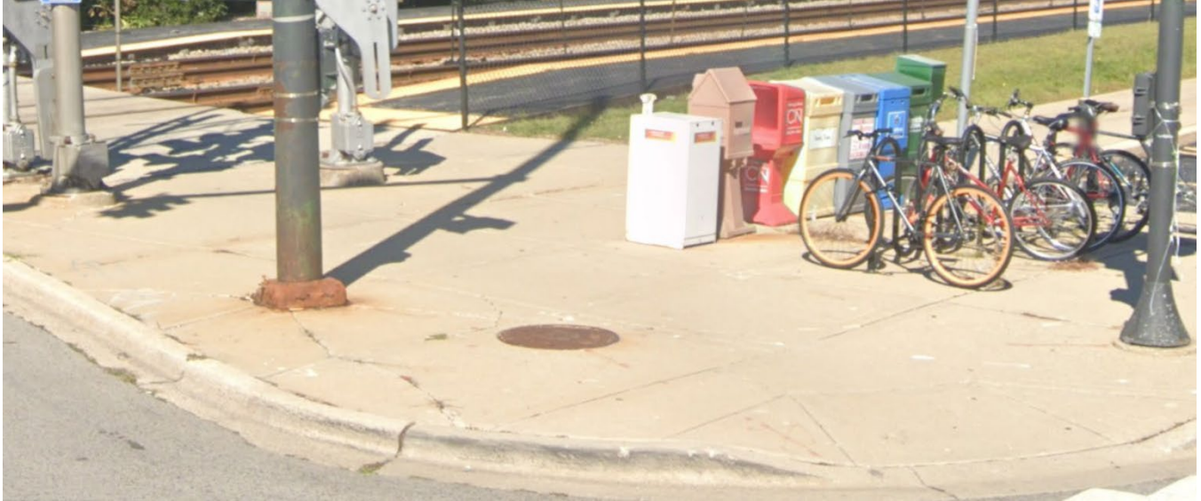
Image 1 (SE portion of Project Area): This access point lacks the proper ADA tactile treatment, and the limited availability of bicycle parking is depicted.
