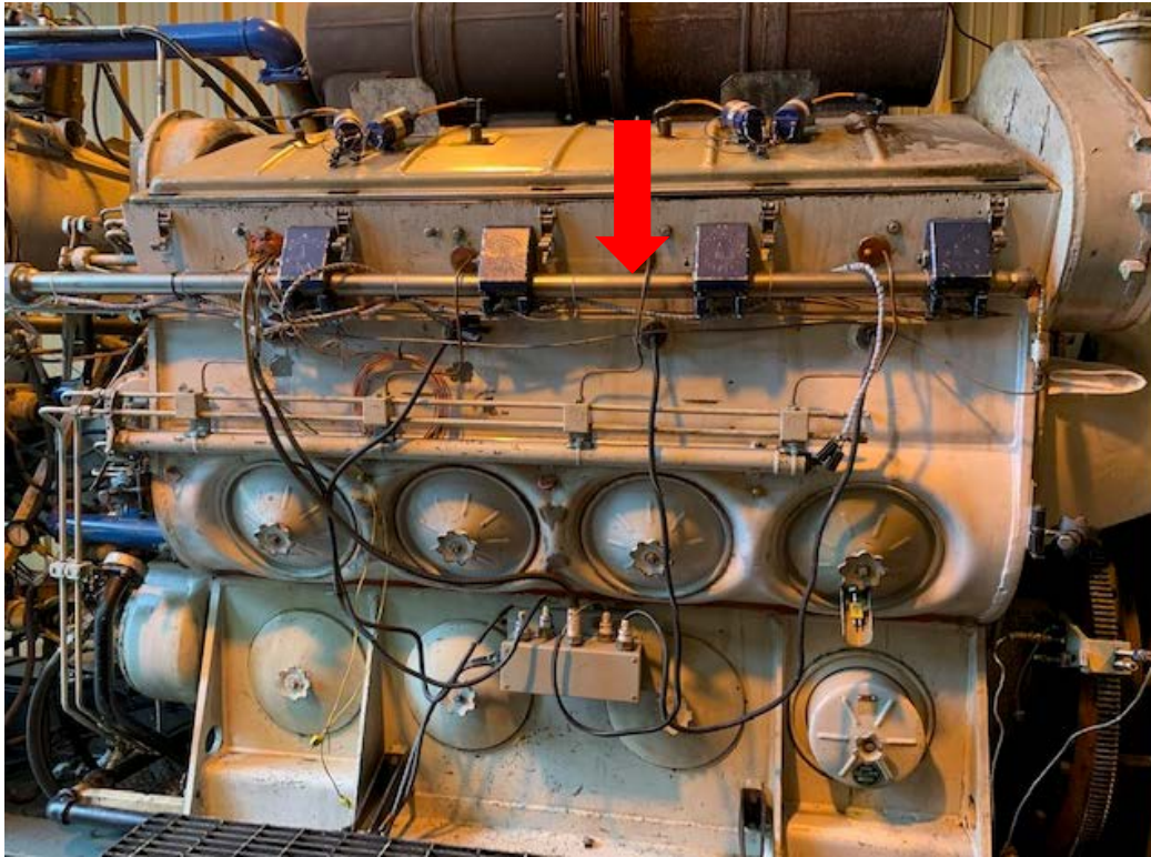
EMD 645 8 Cylinder test engine; gas injection line is pipe running the head.
