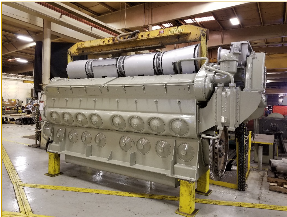
Figure 88 - Typical Two Stroke Turbocharged EMD Engine
