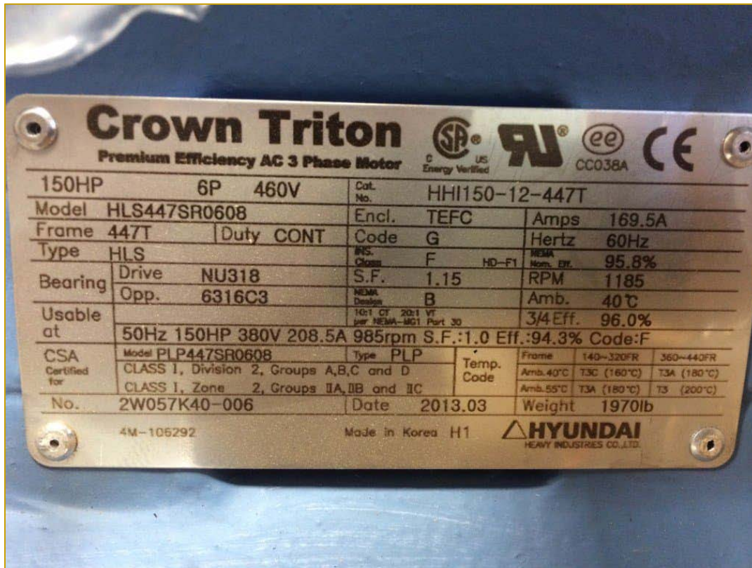
Figure 80 - Example of Class I, Division 2 Rated Motor Nameplate
