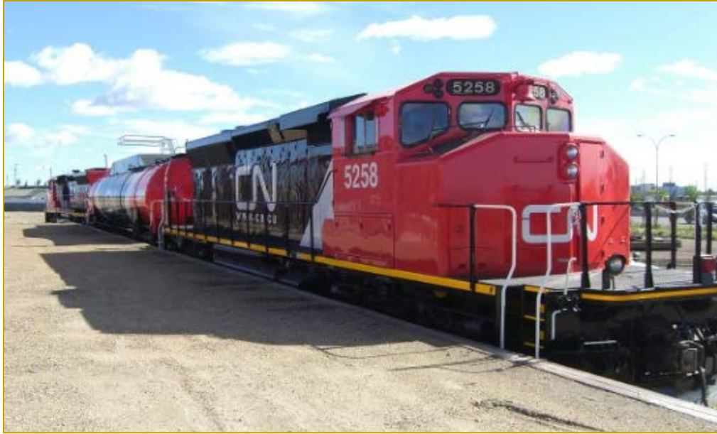
Figure 24 - CN Pilot LNG Dual Fuel Locomotives and Tender Car
