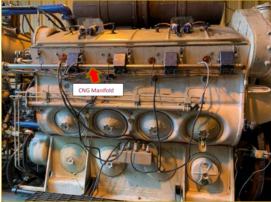
Figure 89 - CNG Dual Fuel Adapted on a Two Stroke EMD Engine
