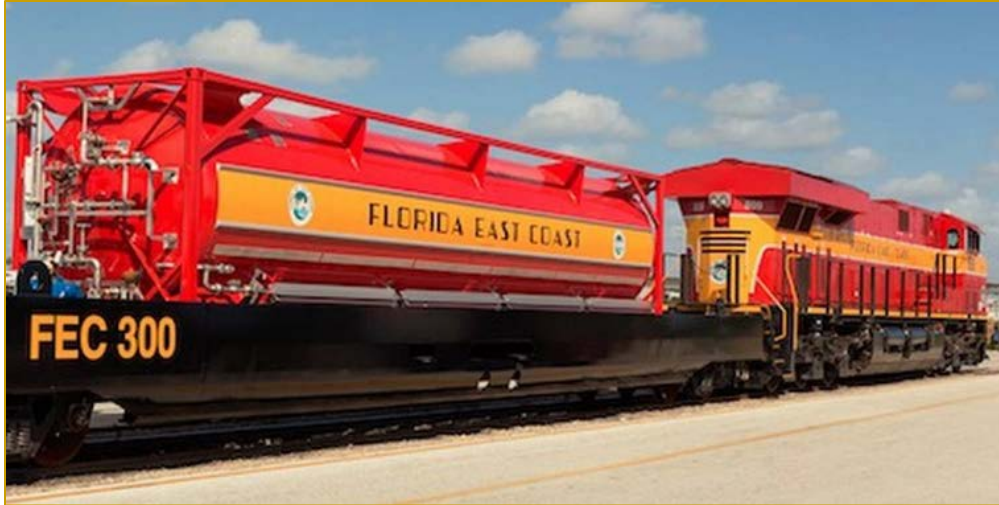
Figure 25 - Florida East Coast LNG Tender Car
