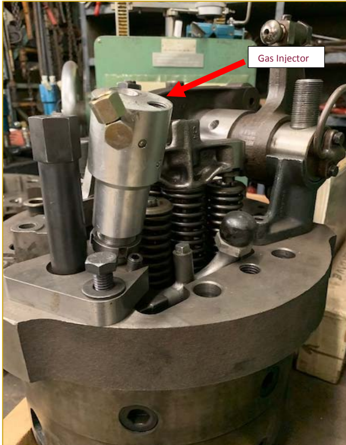
Figure 91 - Cylinder Head with Gas Injector
