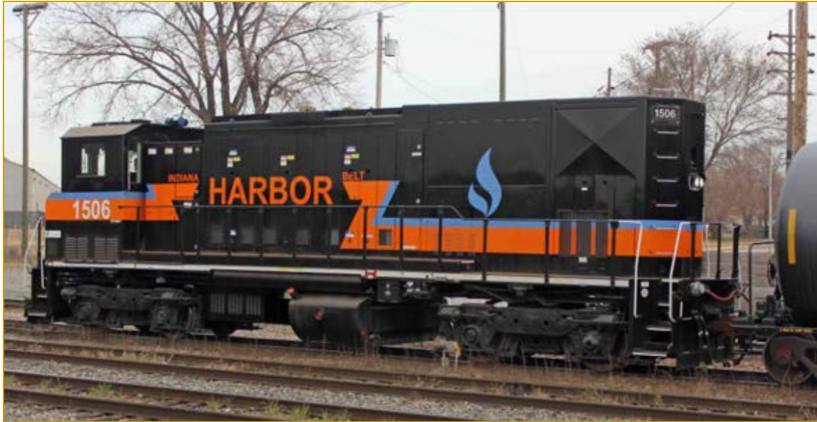
Figure 26 - Indiana Harbor Belt Dual Fuel CNG Switcher
