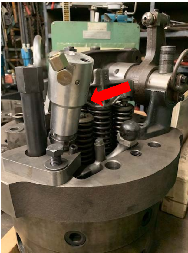
Gas injector installed in the top of EMD power assembly
