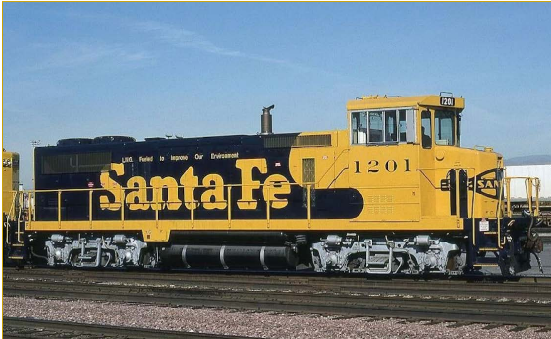
Figure 21 - MK Rail 1200G 100% LNG Powered Switcher
