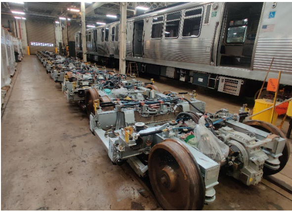
Refurbished truck assemblies waiting to be installed on cars.
