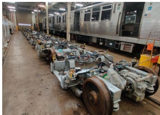
Refurbished truck assemblies ready to be installed on rail cars.
